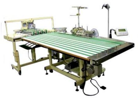
lockstitch Sahl Workstation, with a Re-entry system to attach either flat or folded tape; the tape is automatically cut and ensures that the tape or collar is never twisted. (Less
